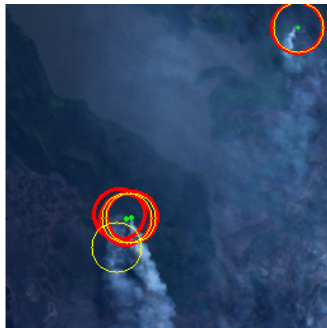
Figure 5. Example of Precision and Recall estimation to a distance threshold equal to 20. There are four predicted fire regions (represented as yellow circles) and four annotated fire regions (represented as red circles).
