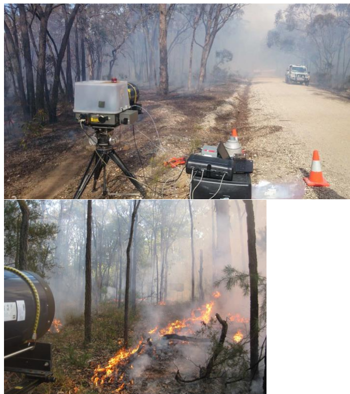
Figure 63: The open-path FTIR instrument set up at a prescribed burn
