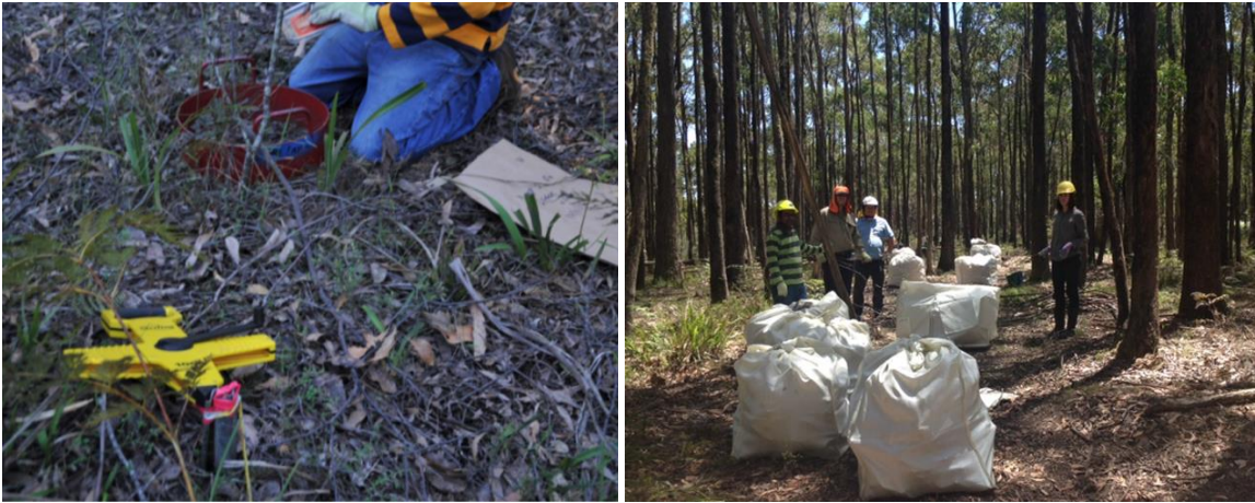
Figure 50: Left) Surface fuels at the fuel source location were assessed to determine in situ fuel hazard level, fuel load and depth). Right) Surface fuels were then raked into large nylon wool bale bags for transport to the Pyrotron. Branch material was similarly collected and put into a wool bale bag for transport
