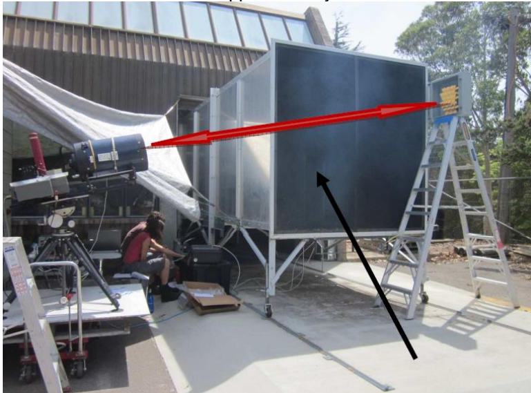
Figure 80: Sampling setup for Pyrotron experiments, in-situ sampling lines (black arrow) and open-path FTIR sampling line (red arrow)
