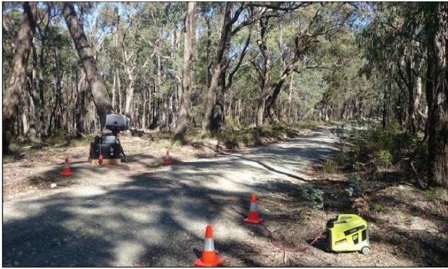
Figure 88 The open-path FTIR instrument was set up along a road.
