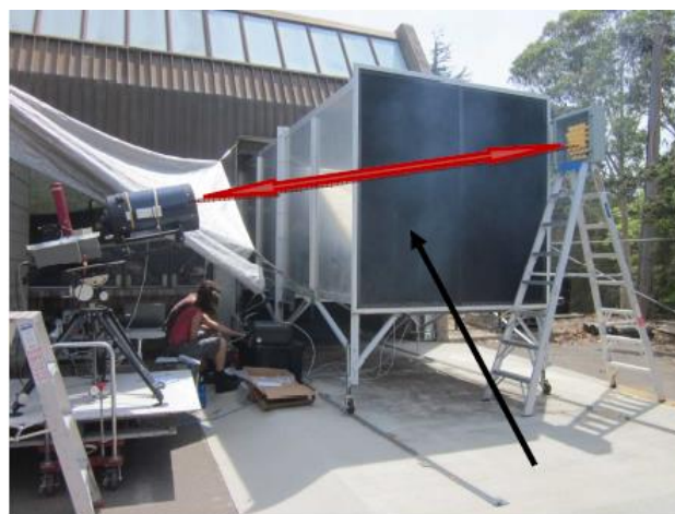
Figure 85 Photograph illustrating the different sampling geometries for the in situ laser spectroscopy measurements and grab sample bags (black arrow) and the open-path FTIR spectroscopy measurements (red arrow).
