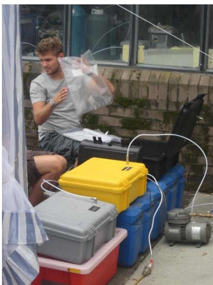
Figure 94: Lung sampling set up to measure Hg emissions for the Pyrotron experiment
