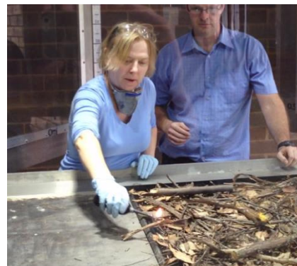
Figure 52: Ignition of the surface fuel occurred via a butane lighter and ethanol in a channel placed on the upwind edge of the fuel bed for heading fires and on the downwind edge of the fuel bed for backing fires.
