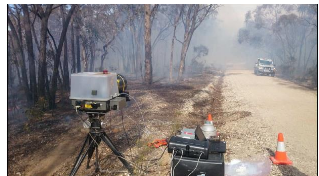
Figure 91 The open-path FTIR instrument was set up along the road
