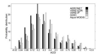
**Figure 4.** Histogram for the matched satellite AOD retrievals and AERONET measurements. The *x* axis shows AOD values and the *y* axis shows the frequency of AOD observations from each sensor relative to the total number of matched AOD observations from the corresponding sensor.
