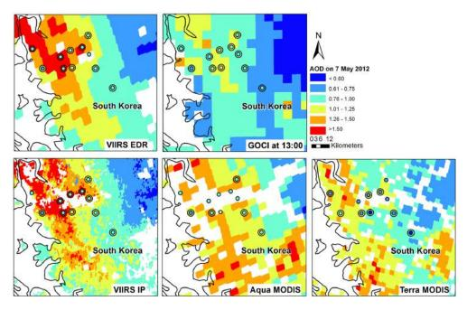
Figure 3. The AOD retrievals at 550 nm from different satellite aerosol products at their designed resolution on 7 May 2012. Coincident Satellite-DRAGON AOD pairs are shown in double circles: the inner circle is the average DRAGON observation within  $\pm 30$  min of satellite overpass and the outer circle is the satellite retrieval that the DRAGON stations falls in.
