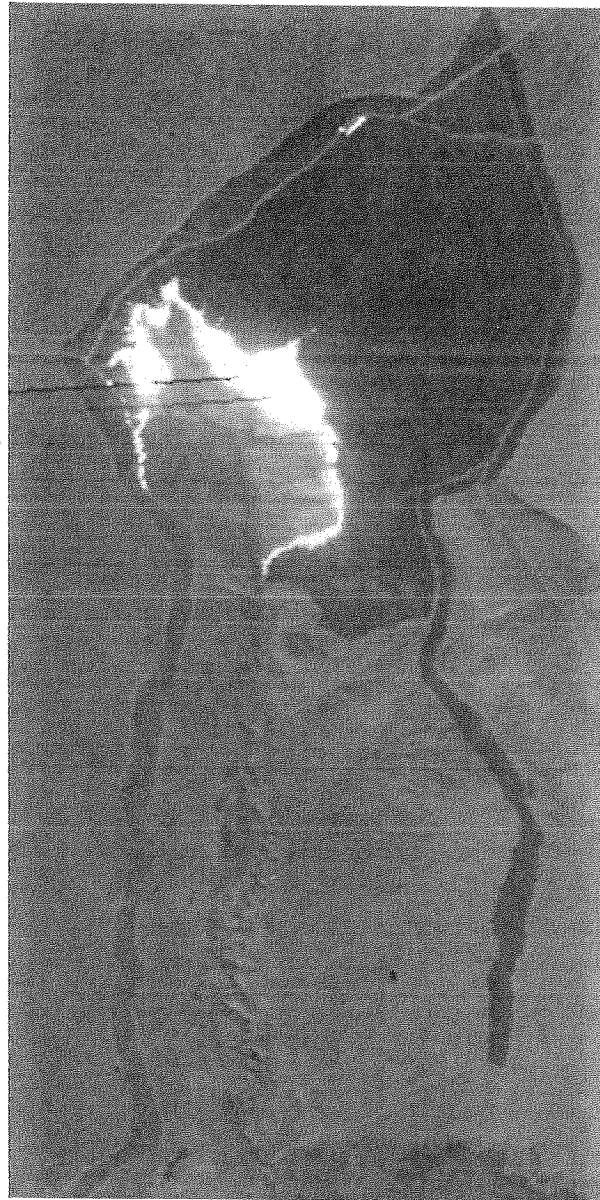
Figure 54.2 AIRDAS image collected over the IBGE ecological reserve near Brasília, Brazil, at 1625 local time. This 1.57–1.70 \mu\text{m} channel displays the active fire in white. The wide portions of the fireline are more intensely burning areas caused by the fire being propagated by the wind.
