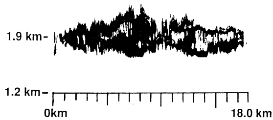
Figure 4.6 Example of LIDAR sounding of the backscatter from smoke particles in a plume from a prescribed fire in southern British Columbia, Canada. New relations provide for the drawing of isopleth lines of equal particulate matter concentration from data collected during a single pass either above or below plumes from biomass fires.
