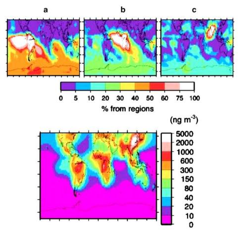
**Fig. 7** (*upper side*) Percent contributions to aerosol BC surface concentrations coming from South American biomass burning (**a**), African biomass burning (**b**) and South Asian industry and residential sources (**c**); (*lower side*) GISS model results for aerosol BC surface concentration (ng m<sup>-3</sup>)
