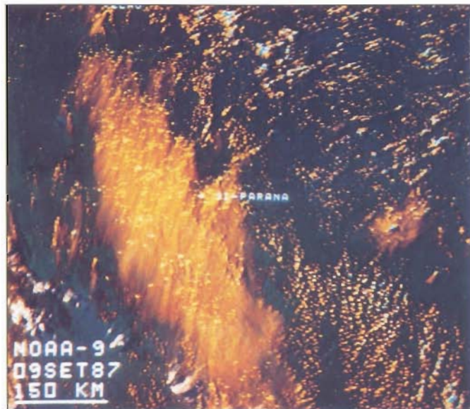
Figure 2B. Smoke emissions from forest and agricultural burnings in the state of Rondonia, Brazil, on September 9, 1987. The yellow cloud shows the smoke produced by the individual fires depicted in Figure 2A. A combination of AVHRR channels one, two and three were used to produce the photo.
